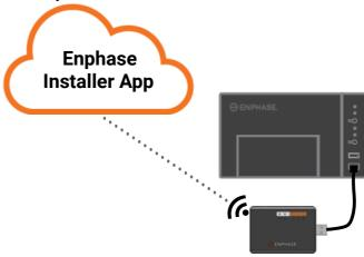
The Enphase Mobile Connect is a modern package that connects to the Enphase Envoy-S or IQ Gateway, and eliminates the need for an on-site Internet connection to monitor an Enphase Microinverter System. The addition of The Enphase Mobile Connect to an Enphase System enables greater installation flexibility and provides reliable system monitoring independent of the Internet service on site.
